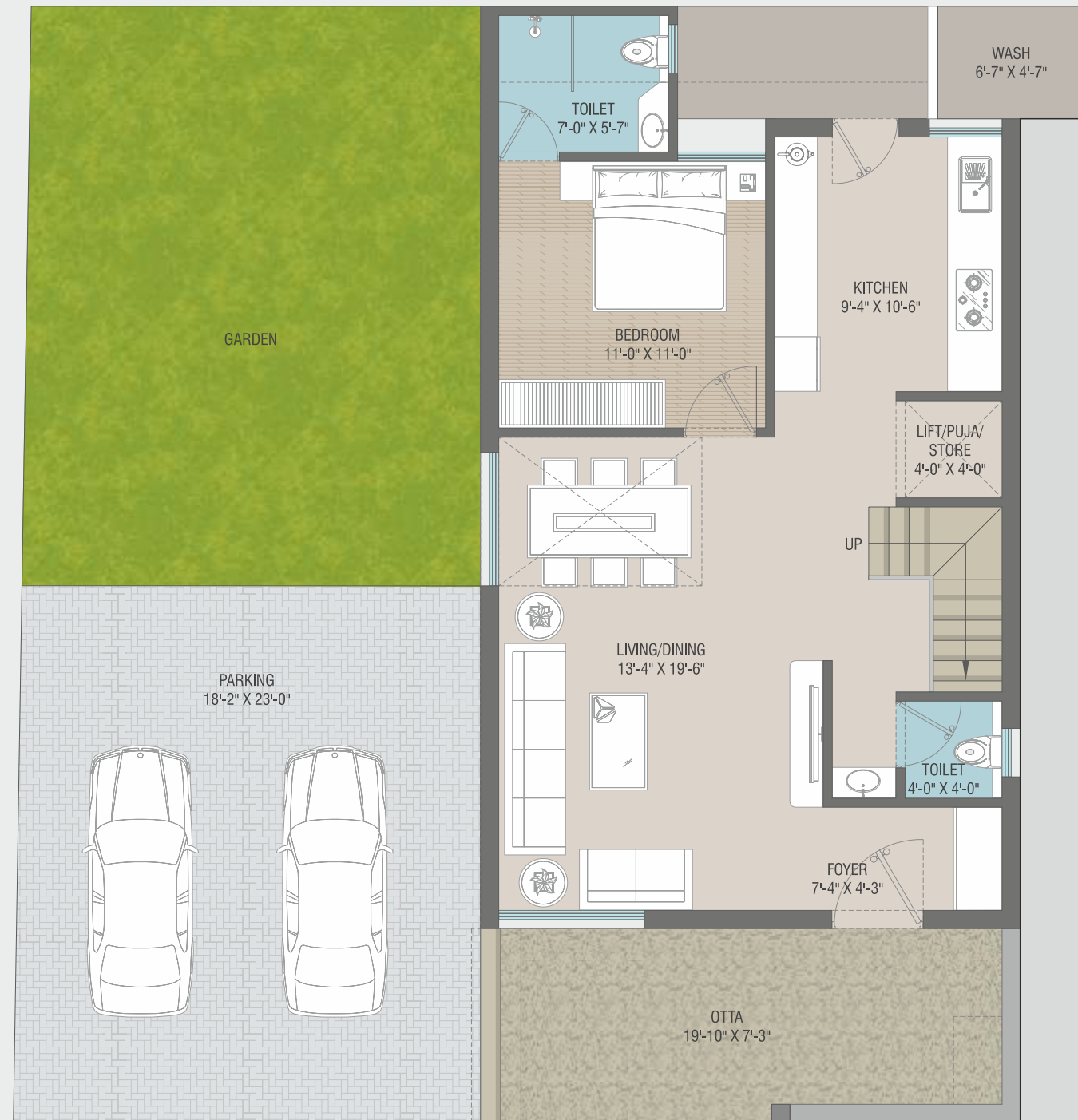
GROUND FLOOR PLAN C.AREA : 681 SQ.FT. BUILTUP : 915 SQ.FT.
