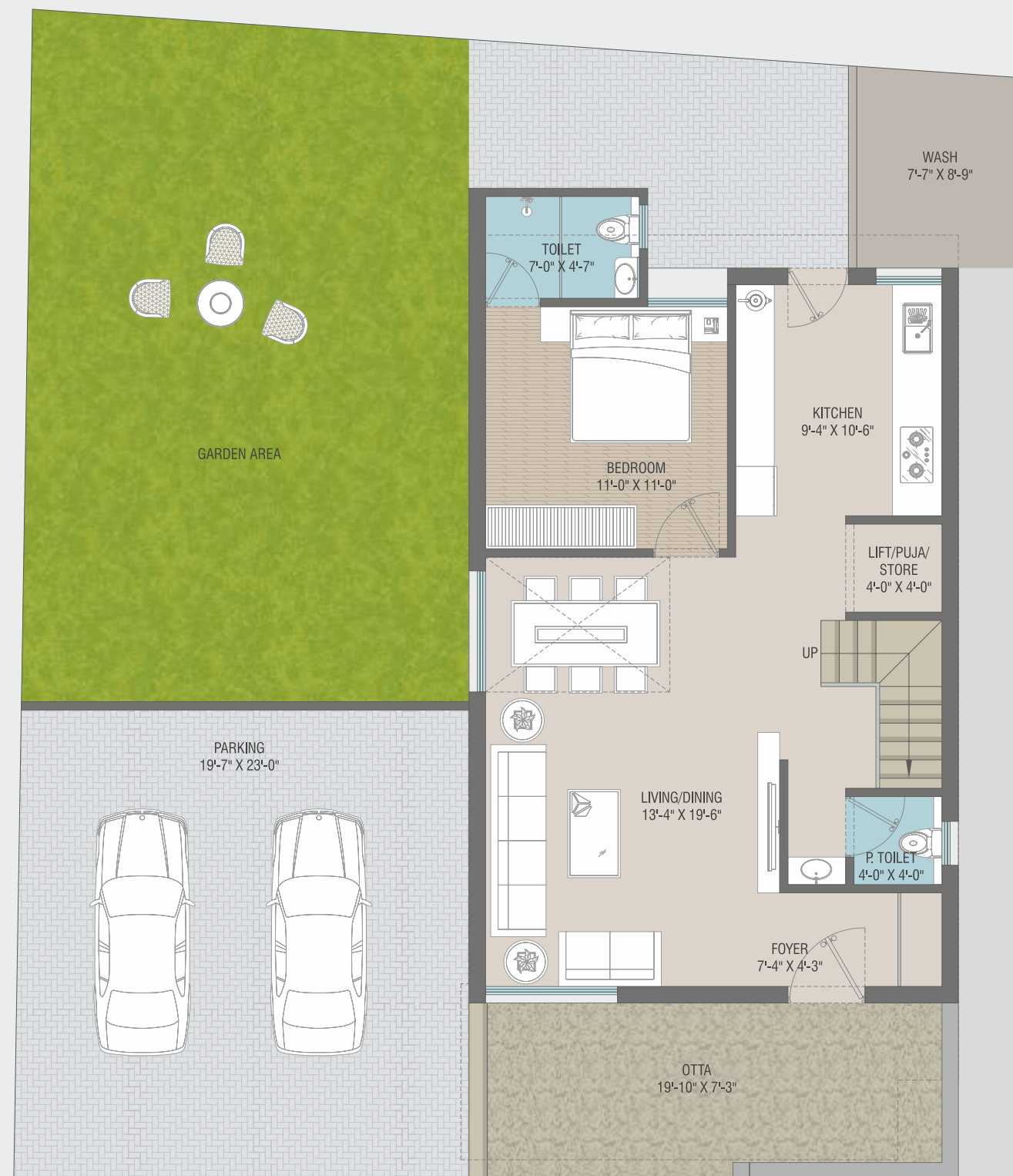
GROUND FLOOR PLAN C.AREA : 674 SQ.FT. BUILTUP : 895 SQ.FT.
